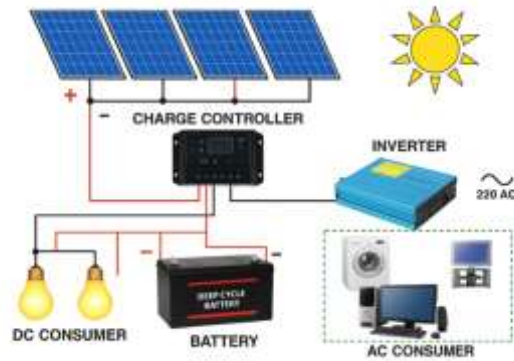
Figure 1. Solar Power System Diagram
