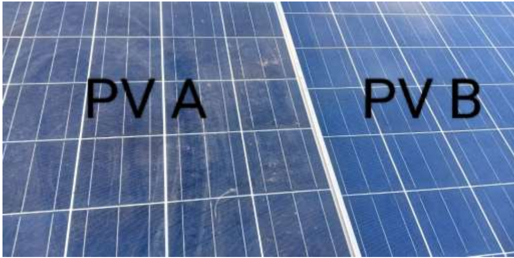
Figure 4. Surface Contamination Images of PV Panels After the Experiment
