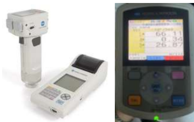
Figure 8 Color Analysis with Minolta CR-400 Chromameter
